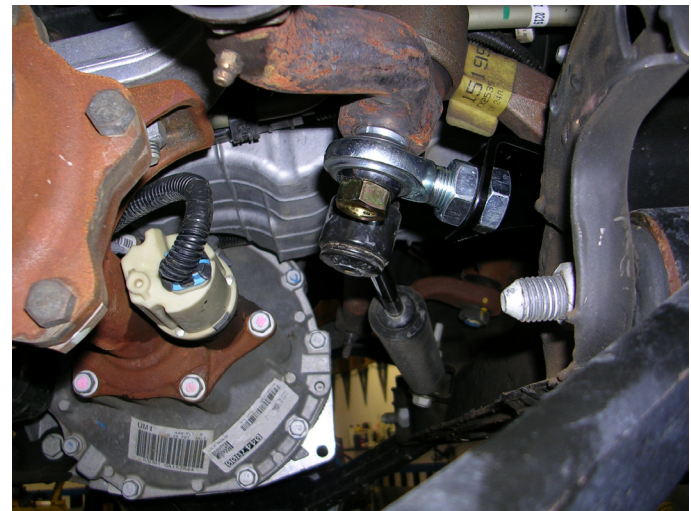
Idler arm bracket installed
