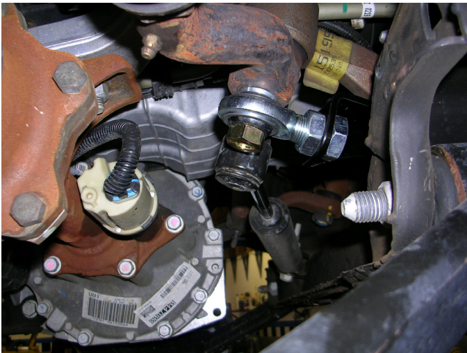
Idler arm bracket installed
