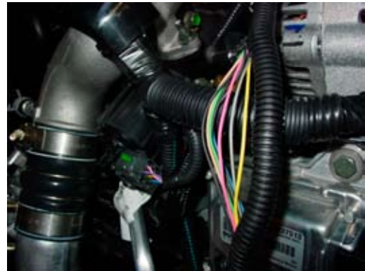
Locate wires to MAF & EGR Solenoid on passenger side front of engine. (may differ for 2006)
