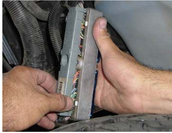
4. Open back of connector by squeezing its sides with your fingers and pulling out.
