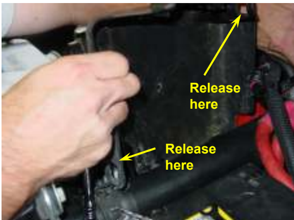
2. Remove plastic cover from PCM by releasing locking tabs as shown
