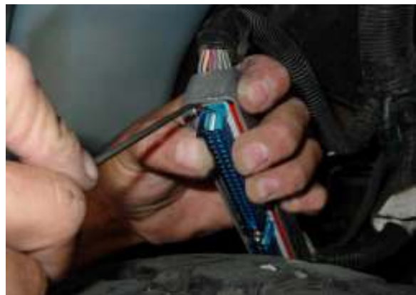
5. Push in white tab on both sides to remove blue connector cover so that pin can be inserted fully.
