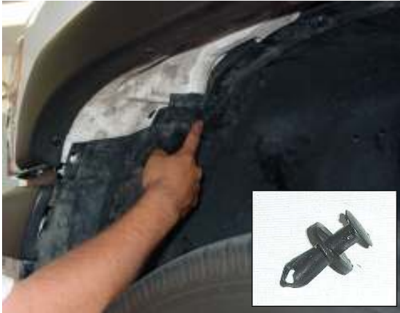
1. Remove wheel-well liner clips on the front left side of the truck wheel-well. Remove wheel-well liner.
