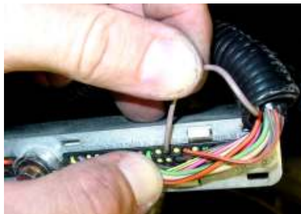
6. Insert auxiliary alternator charge wire in jack #32 on the blue connector.
